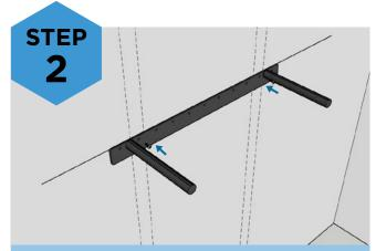
Identify stud locations and ensure screws will attach to a wall stud in at least two locations. Make sure that product is placed in 'THIS SIDE UP' position.
