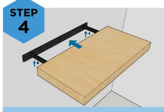
Slide shelf over brackets and install positioning screws into predrilled holes from the bottom in two locations.
