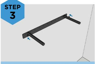
Add additional fastenings in addition to stud locations to ensure there is a fastener in each end of the bracket and maximum spacing between any fastener is 16".
